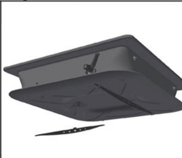
Step 5: (Install Lid to Inlet)
